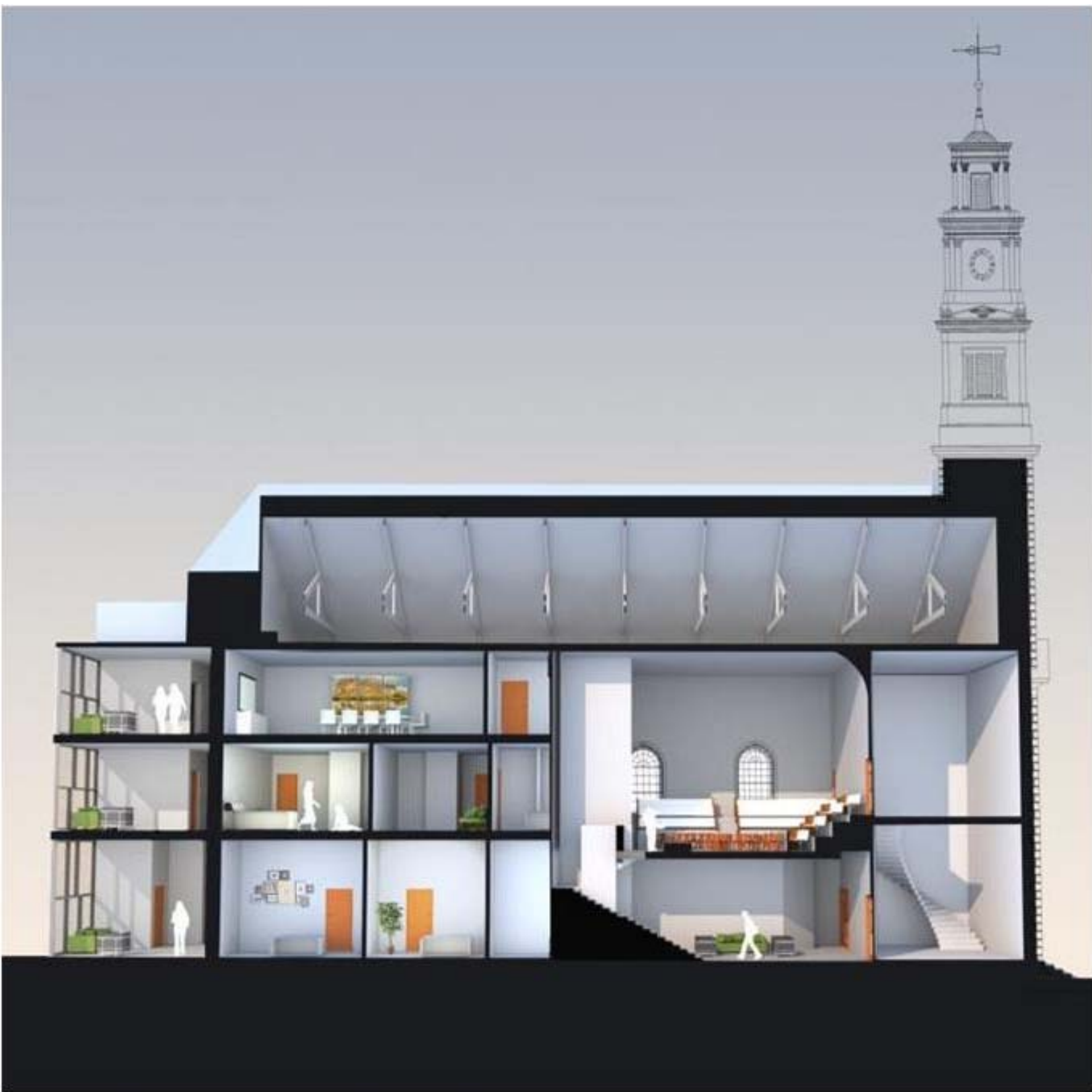
Cross Section of Dina's Dwellings, showing the reconfigured sanctuary space, apartments on the first and second stories and multipurpose space on the third floor. Image used with permission from Jeff Venezia of Design Ideas Group.
